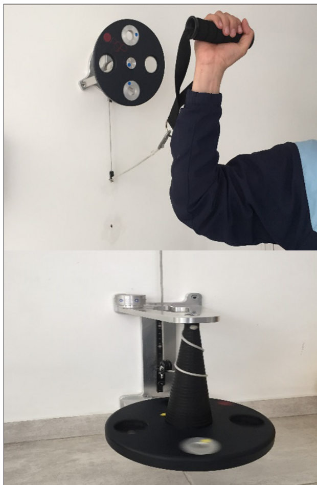
Figure 2 Fixed radius pulley (top) and isoinertial tapered pulley (bottom).
