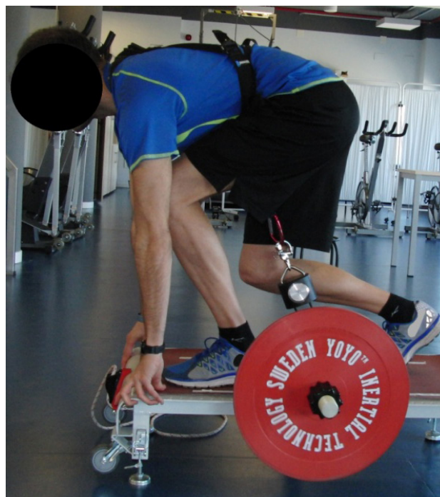
Figure 1 PAPE induction for the lower extremities on an nHANCE™ Squat Ultimate eccentric training machine (YoYo™ Technology AB, Stockholm, Sweden)
